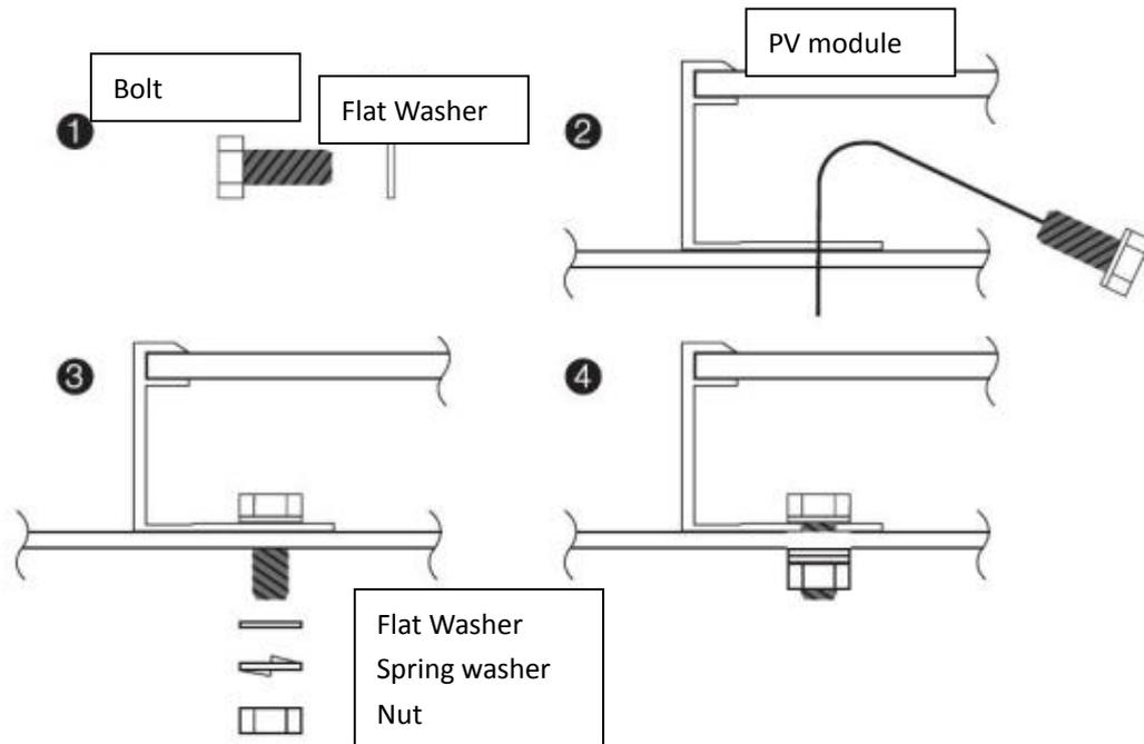
**Figure 2 Installation Method**
