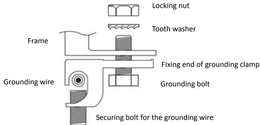
**Figure 7 Installation Method**
