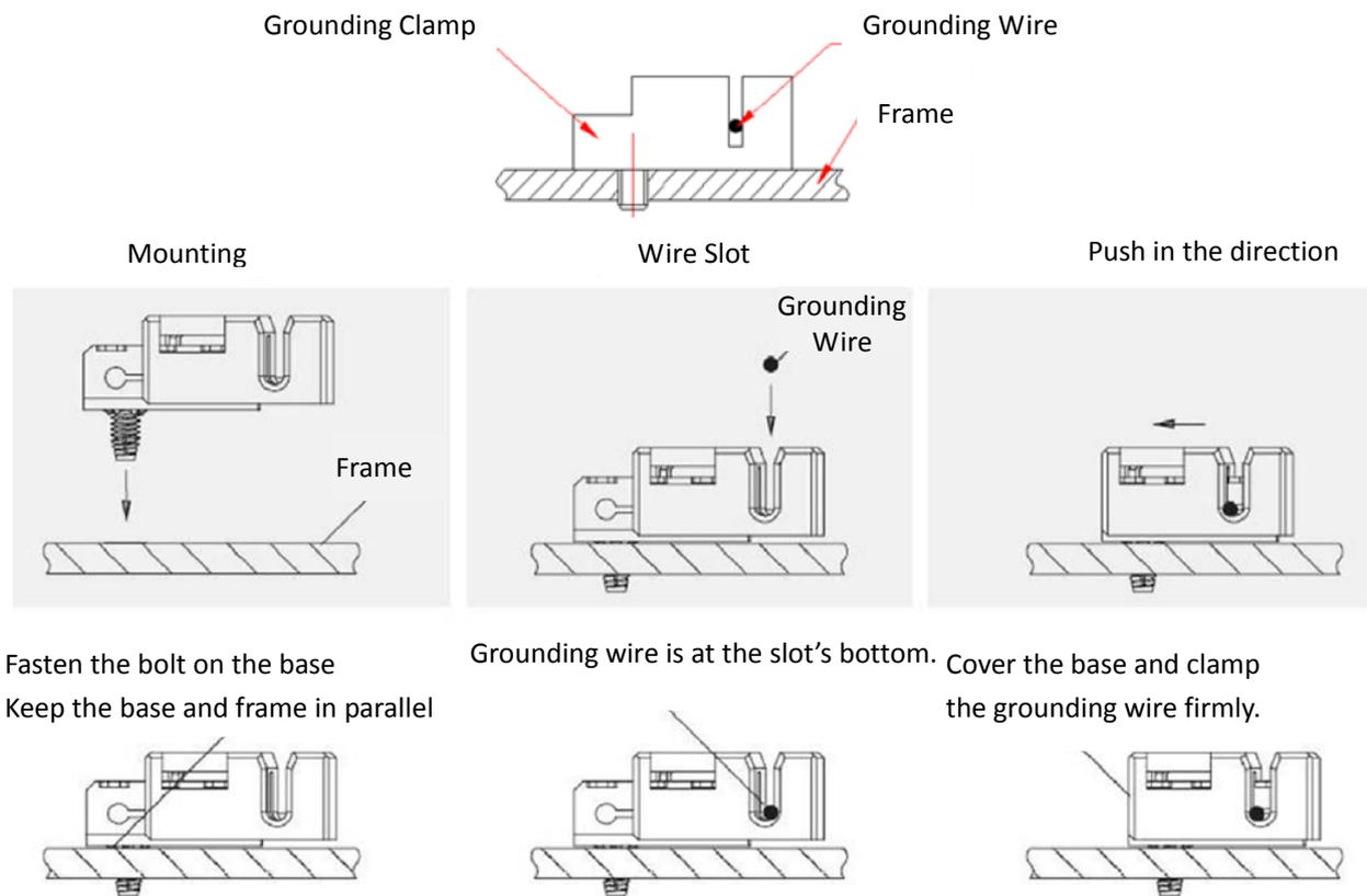
**Figure 6 Installation of Grounding Clamp**
